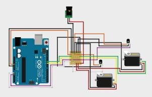
A magnet was embedded in the horn of each servo, and a hall effect sensor is mounted on each servo horn so it is a few millimeters above the magnet. By pushing on the horn, the magnet moves relative to the sensor proportional to the force applied.
